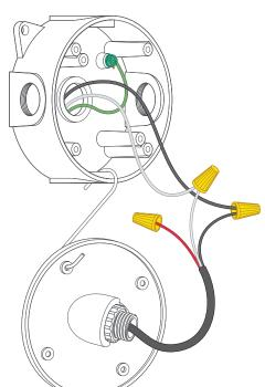
Use the included wire nuts to secure and protect the connections.
