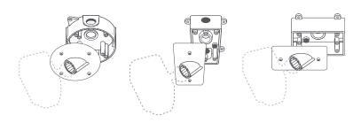
Ensure that the electrical box you use is weatherproof, including threaded plugs. Use sealant if necessary.
